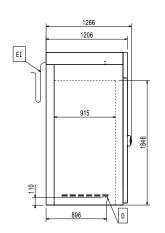
CWII Cold Water inlet 1 (cleaning) Drain D
